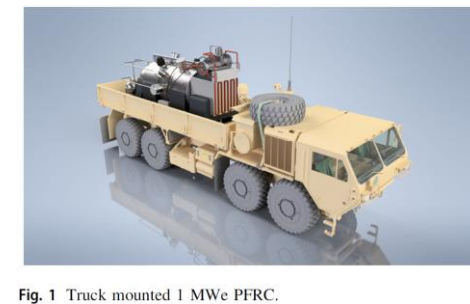
Fig. 1 Truck mounted 1 MWe PFRC.
