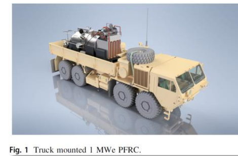
Fig. 1 Truck mounted 1 MWe PFRC.
